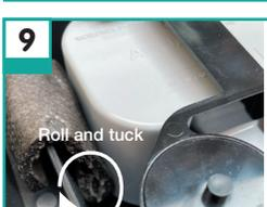
Tightly roll **both** inside ends of the capillary matting and tuck into the AQUAbox alongside the AQUAvalve.
